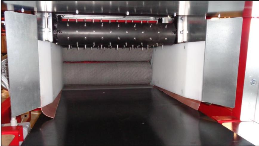
Regularly inspect the fiber bale infeed assembly for damage. There are two spiked pinch rollers utilized in this assembly. A damaged pinch roller can cause an improper soil mix. If the spikes are damaged or missing, repair or replace the roller(s) immediately. Contact the manufacturer for all replacement parts.
