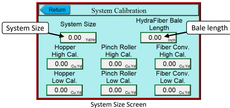
6. Enter line volume into “System Size” field. **Note:** this machine is rated up to 25 Yds/Hr.
